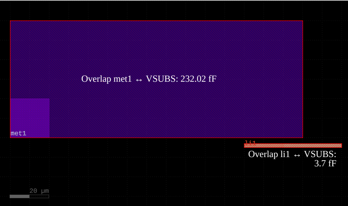
Figure 24: Overlap capacitances to substrate.
